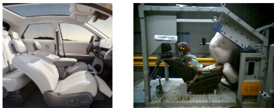
Figure 1 Reclined seat and sled test for a reclined sitting position
