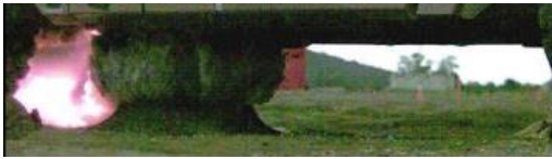
Figure 2: Initial blast loading impacting the vehicle.
